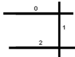
Figure 1: Line diagram to be represented in BSP Tree. Lines should be added to the tree in the order 0, 1, 2.
